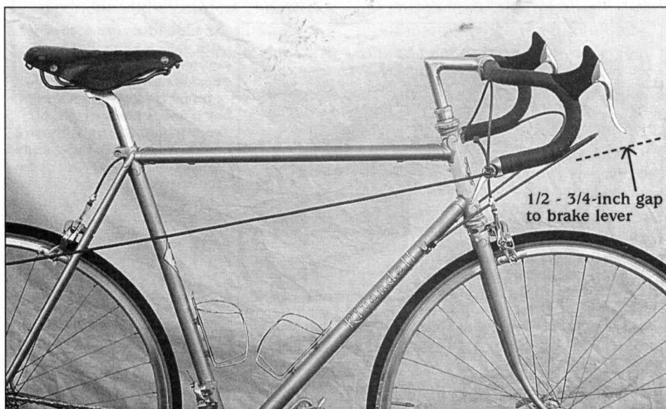
Profile of a Dream bar, with a normal/classic 23 degree ramp, 140mm drop, and 90mm reach.
