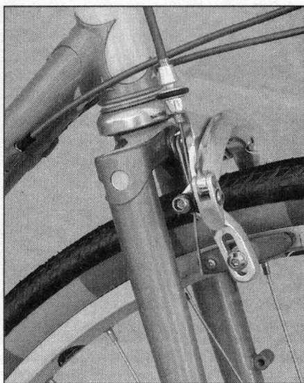
Bottom head lug & fork crown detail.
