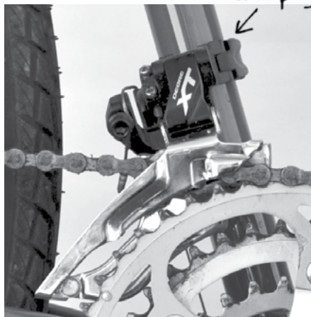
Brazed-on front derailleurs: one of the all-time worst ideas (in bikes)
