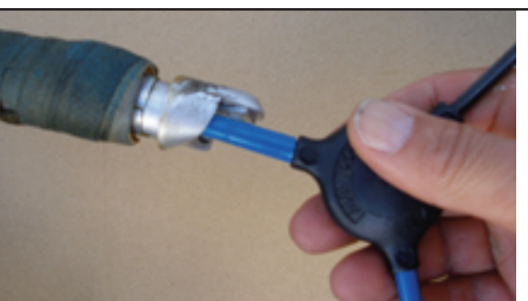
8. Loosen expanding bolt, extract pod.
