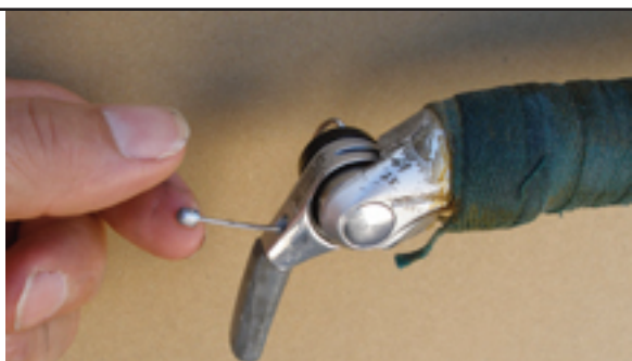
5. Pull out the cable. Reuse it, fine.
