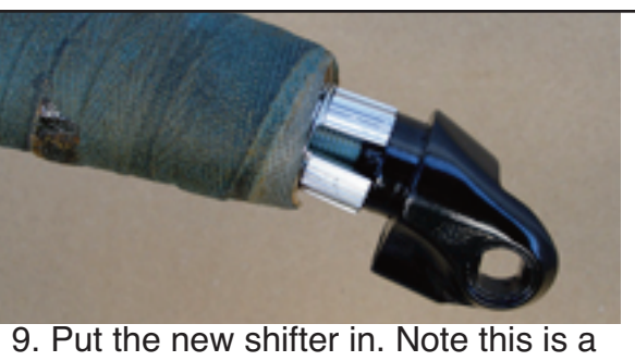
9. Put the new shifter in. Note this is a front bring used as a rear. Friction shifting doesn't care. Tighten it.
