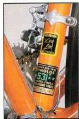
Campagnolo derailleur system and versatile 14-16-18-21-24 Regina rear cluster with 42-52 chainwheels.
