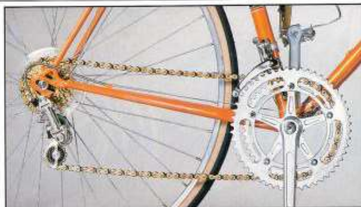
Campagnolo derailleur system and versatile 14-16-18-21-24 Regina rear cluster with 42-52 chainwheels.
