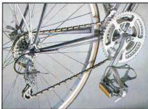
SunTour Cyclone front and rear derailleurs on this remarkable touring machine.
