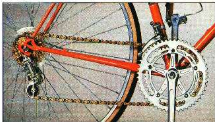
Campagnolo derailleur system and versatile 14-16-18-21-24 Regina rear cluster with 42-52 chainrings.
