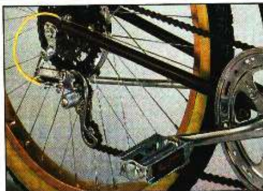
5-speed Sidewinder includes a 14-17-22-28-38 rear cog and a Sun Tour AG rear derailleur.
