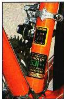
Campagnolo derailleur system and versatile 14-16-18-21-24 Regina rear cluster with 42-52 chainrings.
