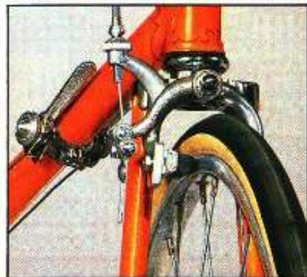
The bike's Campagnolo caliper brakes are matched to 700C Super Champion rims and Schwinn Super 700 250g tires.
