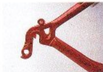
Our patent-pending G-Force chainstays virtually eliminate chain slap, while the vertical dropouts keep the rear axle from shifting under load.
