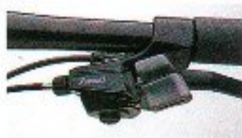
The Shimano Rapid-Fire Shifter lets you change gears quickly and accurately with just a flick of your thumb.
