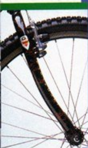
The PDG OS "Super-Lite" G-Force Fork with unique, internal butting and continuously curved design for superior shock absorption.
