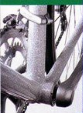
The Series 5 uses a unique, flared seat tube that decreases bottom bracket flex more than conventional round seat tubes.
