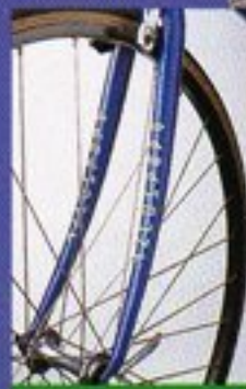
The Tange Butted Chrome-Moly Unicrown Fork: one of the lightest, most durable forks to be found on any road bike at any price.
