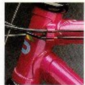
Integral cable guides are part of Paramount's investment-cast custom lugs. Result: cleaner butts in the tubes, lighter weight and greater strength in the frame.
