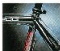
Very clean: "macaroni" cable routing.
