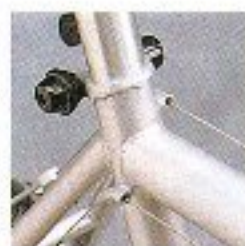
Clean: investment-cast seat collar with integrated cable routing for brake and derailleur.
