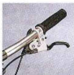
Exage LT components include Rapidfire Plus, Dual SIS, Multi-Condition brakes.
