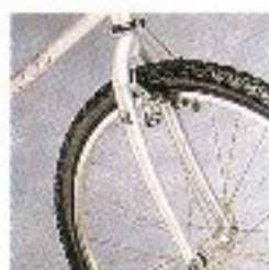
Competitive edge: Short-rake fork design complements a steeper head angle for quicker handling through technical sections. Improved stability at speed. Note continuous and taper fork blades.
