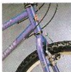
Avenger OS headset, Araya VP-20 rims stand up to the rigors of serious off-road use.
