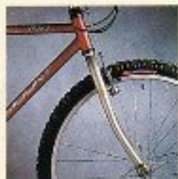
Power Steering: Fast-handling 71.5° head angle with 38mm reduced-rake fork for improved stability.
