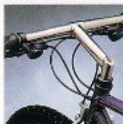
What's Up Front that Counts: Ritchey Force bar and d/b CrMo stem. Both with Satin Titanium finish.
