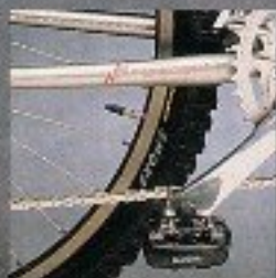
Details, Details, Details: Smoke/Dart folding tires, ultra-hard anodized finish CR-16 rims, double-buttet Wheelsmith spokes, red alloy nipples.
