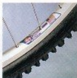
Quad Construction: 32" doublewall CR-16 rims, WheelSmith spokes, Smoke/Dart tires.
