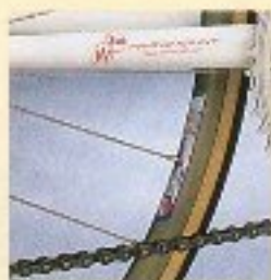
Quad-Built Precision: Sun Metal M14A rims, Wheelsmith 15 gauge SS spokes, Vivezza racing tires.
