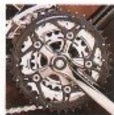
Shimano STX 21 speed component group with compact crankset.
