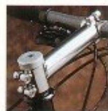
Exclusive Quad Tech 427 Stem with four different positions.
