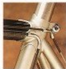
Cable routing system for tight, clean design.
