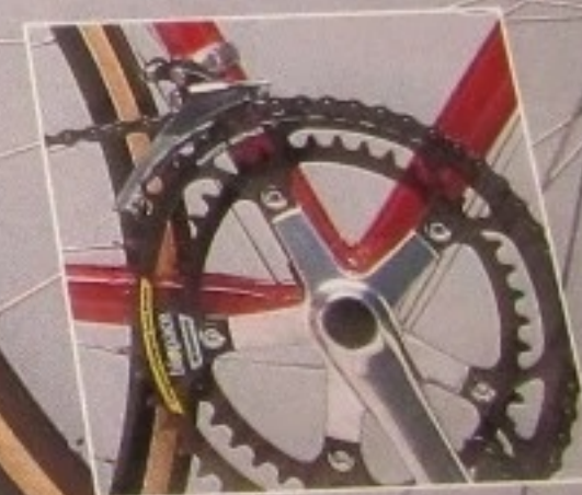
Shimano Biopace chainwheels maximize pedaling efficiency.
