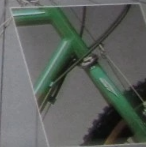
Uni-crown fork with New Shimano Deore front brakes
