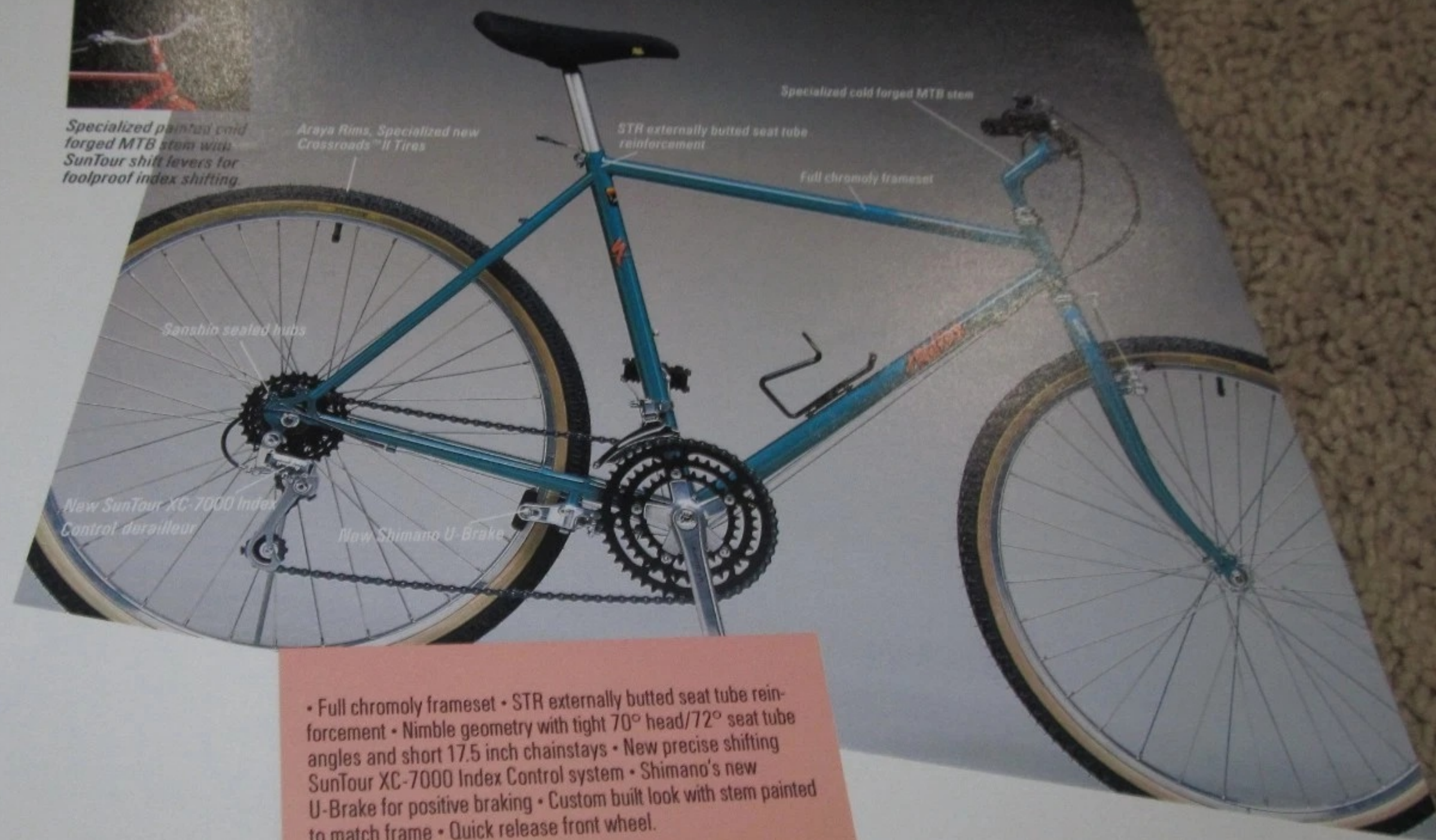
SunTour XC-7000 Index Control derailleur with 13-30 tooth wide range freewheel.
