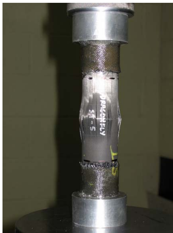
Figure 11. Hy-Bor Seat Tube After Compression Testing
