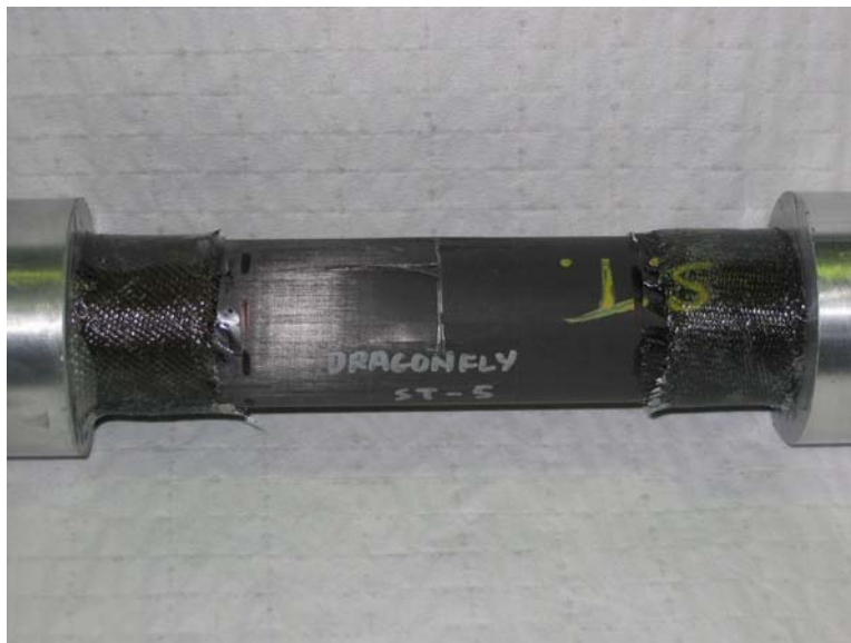
Figure 10. Hy-Bor Seat Tube After Impact Damage
