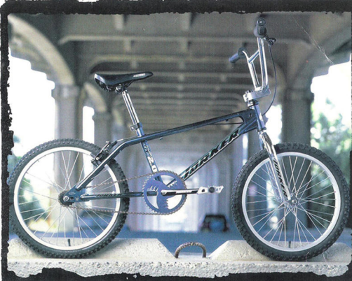
TR2.0 If you're tired of tearin' up cheap bikes that your mom buys you at the department doesn't ask questions. It's got a threadless headset, alloy platform pedals with chromoly axles
