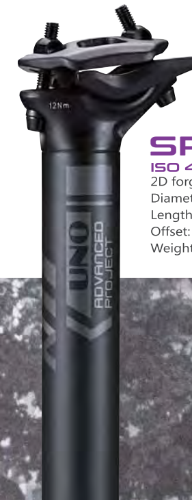
SPF2015 ISO 4210 - R/M approved 2D forged head, 2014-T6 shaft Diameter: 27.2/30.9/31.6mm Length: 300/350/400mm Offset: 0mm Weight: 260g(31.6mmx350mm)
