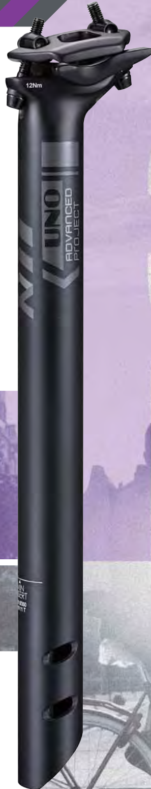
SP729 ISO 4210 - R/M approved 3D forged one-piece, 7050-T6 shaft Diameter: 27.2/30.9/31.6mm Length: 300/350/400mm Offset: 10mm Weight: 277g(31.6mmx350mm)
