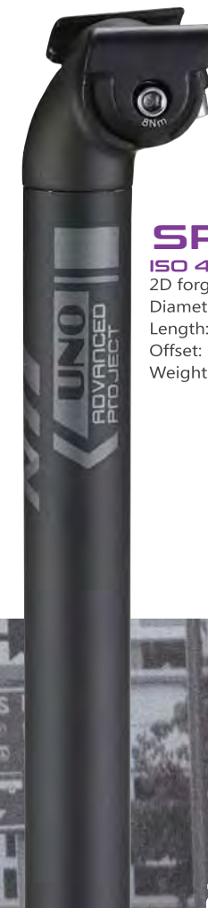
SP629 ISO 4210 - R/M approved 2D forged head, 2014-T6 shaft Diameter: 27.2/30.9/31.6mm Length: 300/350mm Offset: 10mm Weight: 287g(31.6mmx350mm)
