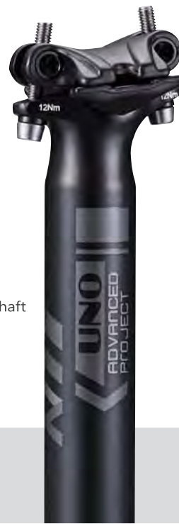
SP376 ISO 4210 - R/M approved 3D forged one-piece, 2014-T6 oval shaft Diameter: 27.2/30.9/31.6mm Length: 300/350/400mm Offset: 25mm Weight: 307g(31.6mmx350mm)
