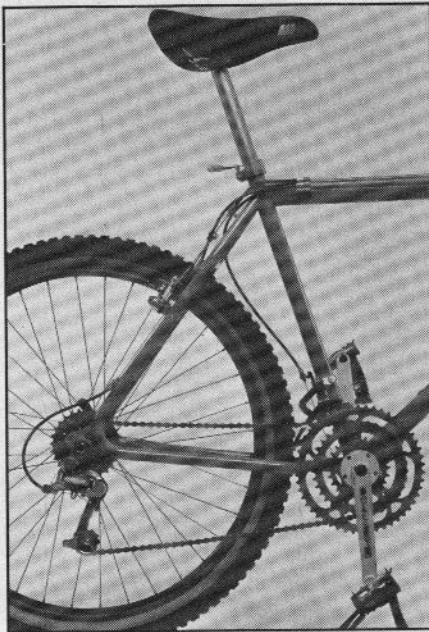
A special computerized tube bender is used to form Yeti's one-piece rear triangle.
