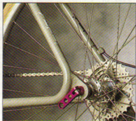
The A.R.C.'s one-piece, computer-bent stays apply a traditional Yeti design to thin aluminum tubing.
