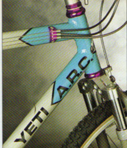
Easton's Varilite tubing is so thin that the cable guides are riveted—which adds no heat stress.
