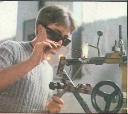
Brazing of fittings Inspection of brazed parts by liquid penetrant
