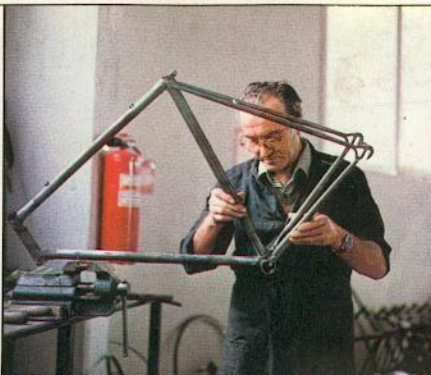
Visual inspection of frames after welding
