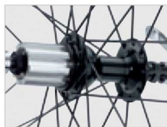
Hubs with traditional flanges mounted on Hi-Precision bearings, G3 spoking
