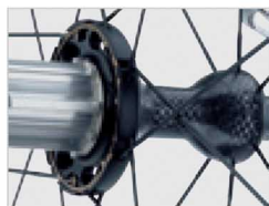
Rear hub in structural carbon with variable thickness, with oversize flange
