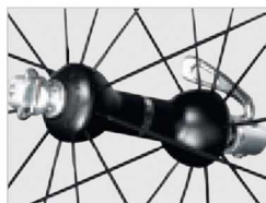
Record-class aluminium HPW front hub
