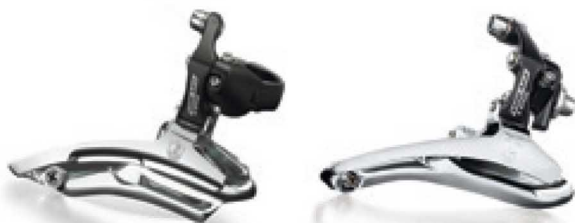
Mirage front derailleur, available in the braze-on or Ø 28,6 and 32 mm clamp-on versions for double and triple drivetrains
