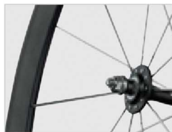
High-profile rim with 20-hole spoking on the front and 24-hole spoking on the rear
