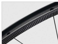
Structural carbon rim for clincher tire
