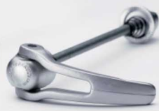
New quick release, 21 g lighter than the preceding version. The lever is in cold-forged aluminium and has two pivots for more balanced clamping.
