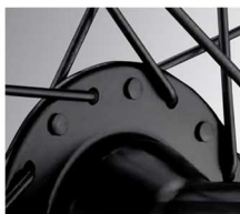
STRAIGHT-HEAD SPOKES: maximum stiffness of the wheel – maintains performance over time.
