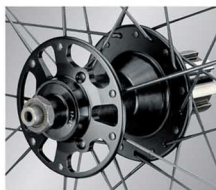
OVERSIZE FLANGES: make it possible to obtain greater torsional stiffness, increasing the overall reactivity of the wheels.
