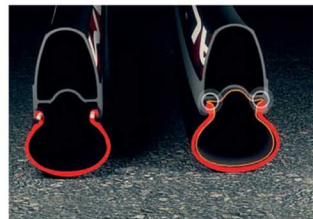
The tubeless tire does not have an inner tube and consequently there is no risk of sudden deflation due to punctures.
