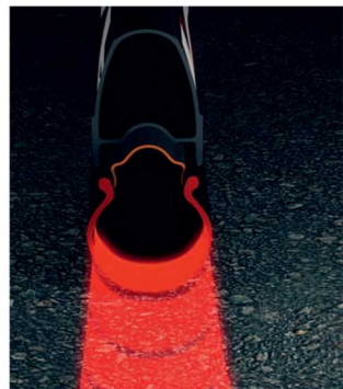
The tubeless tire rolls more smoothly thanks to the absence of friction between tire and inner tube.
