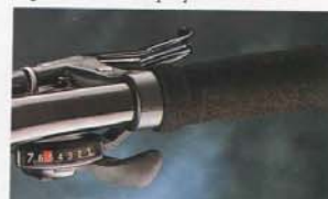
STX Rapidfire Plus gear shifters with Optical Gear Display
