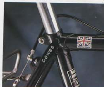
Seat cluster with internal cable routing, and oversized seat post - for increased rigidity.
