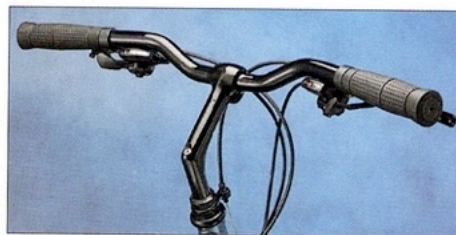
'Low rise' bars provide a comfortable riding position.
