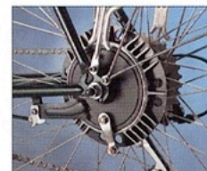
Arai drum rear brake for assured stopping power.
