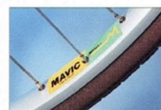
Mavic tandem 40 hole anodised rims for perfect balance, strength and lightness.
