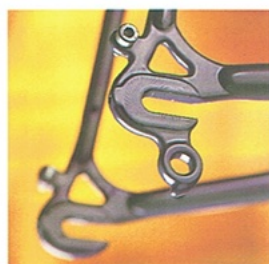
Forged rear drop-outs with mudguard fitting
