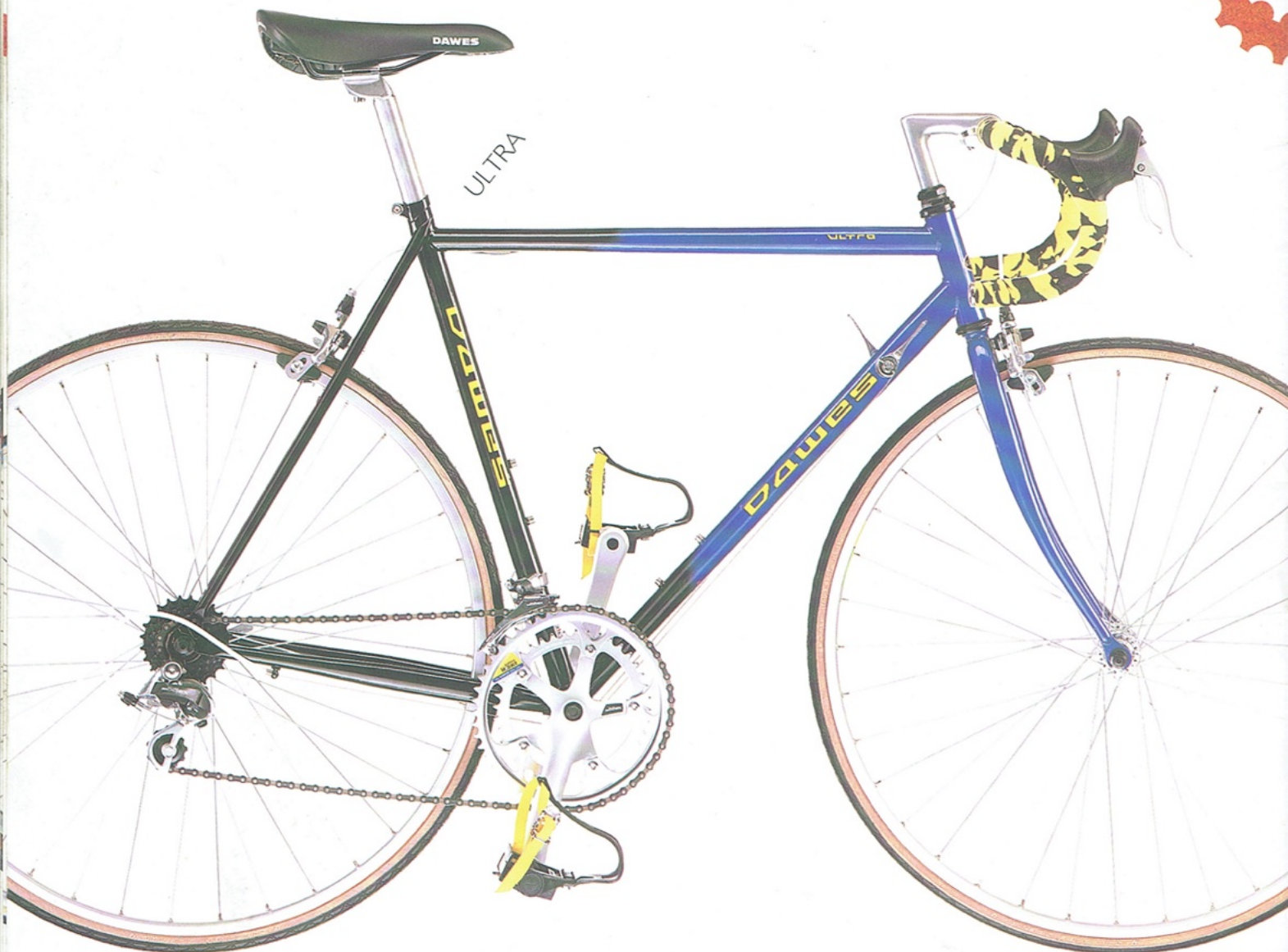
Elliptical tubing and tig welding featured within the race range
