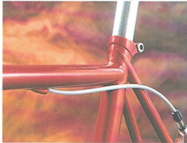
Elliptical tubing and tig welding featured within the race range
