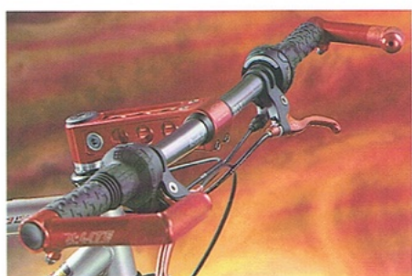
Handlebar assembly featuring Exlite, Renthal and Sachs components
