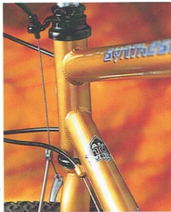
AM-10 tig welded frame
