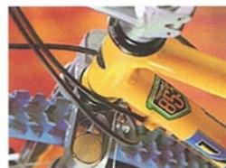
Frame featuring the new Reynolds 853 fillet brazed tube set
