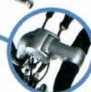
Trafficflex suspension stem
