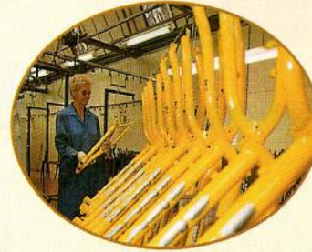
Under the watchful eye of Barbara, each Dawes frame is provided with its ultra-tough Damage Limitation polyester finish.
