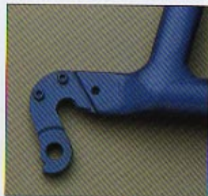
Our new, replaceable rear derailleur hanger can turn a major expense into a minor inconvenience. Photo by Frank Poole.
