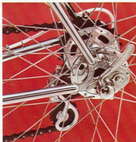
Simplex rear ends of the PX 10 E.
