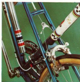
On this picture you see the special mounting of the Mafac rear brake.
