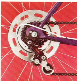
Simplex Prestige rear derailleur and spoke protector.
