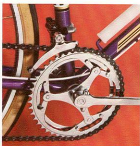
Front derailleur and chainwheels of the AO 8.
