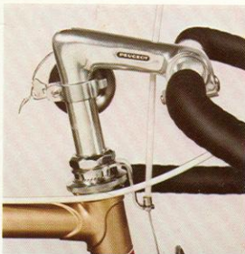
Special Peugeot Philippe handlebar. You see the Simplex Competition ballhead fitting too.
